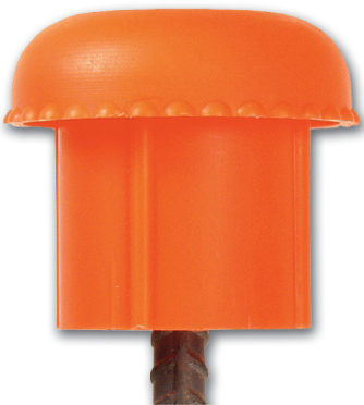
Rebar "bump" cap (also known as "mushroom cap"). Not used for impalement protection.
